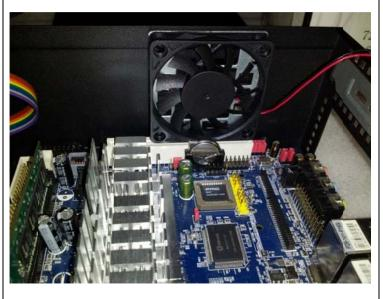
add-on card cannot be used when fan is in place.
