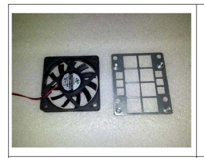
1. Install DD-S21-60BRT bracket onto a 60mm fan.
