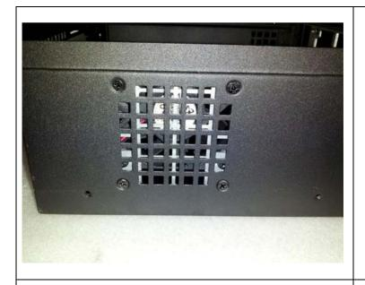
4. Secure fan bracket onto chassis with 4 screws from outside of chassis.
