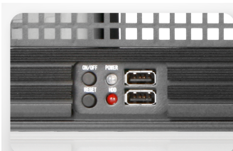
2x USB 2.0 Power HDD LED indicators power reset switch
